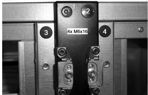
Figure 23 – Centre pillar replacement
