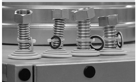
Figure 11 – Connection of heat-exchangers (cap nuts)
