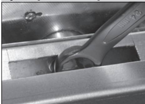
Figure 7 – Tighten the shaft bolt using wrench # 24
