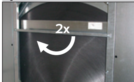
Figure 2 – Rotor Fixation Removal
