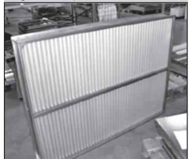
Figure 2b - Drop eliminator
